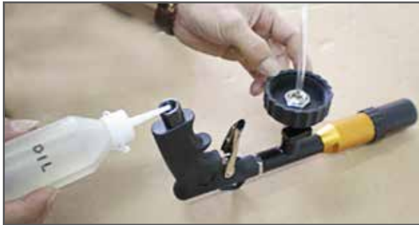
When the aluminium tube doesn't rotate, spray some lubricant WD40 or other brand into in the air inlet.
