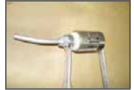
Hold the motor with spanner 11mm and 7mm to loosen the aluminium tube
