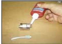
Apply some Loctite before mounting the new aluminium tube.
