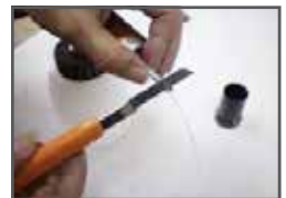
Cut the teflon to the same length as the curved metal tube
