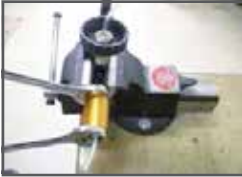
Unscrew the nozzle and loosen the motor housing
