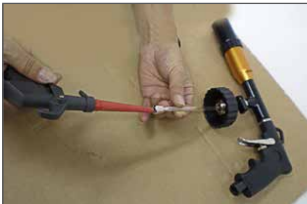
When your Modern PIK Cleaning Gun doesn't aspirate any product, blow air through the filter in the metal weight of the flexible tube
