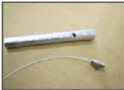
To remove teflon kit you need 11 mm box spanner
