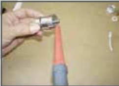
Blow out the motor housing on both sides with air.
